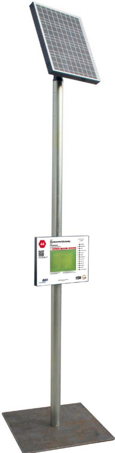
The MOFIS® MEDIA.ECO Timetable provides the capability to display static timetables electronically. A bi-stable cholesteric LCD display with a resolution of 640 x 480 pixels doesn't need any power supply for a static illumination. Display updates are accomplished via GSM / GPRS.
